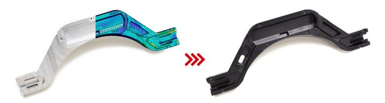
Aluminum bracket with half FEA analysis (left) and KyronMAX® final molded part (right). The FEA analysis is used to translate a metal part into a lightweight plastic molded part, while matching or exceeding the strength and stiffness of the original metal part.
