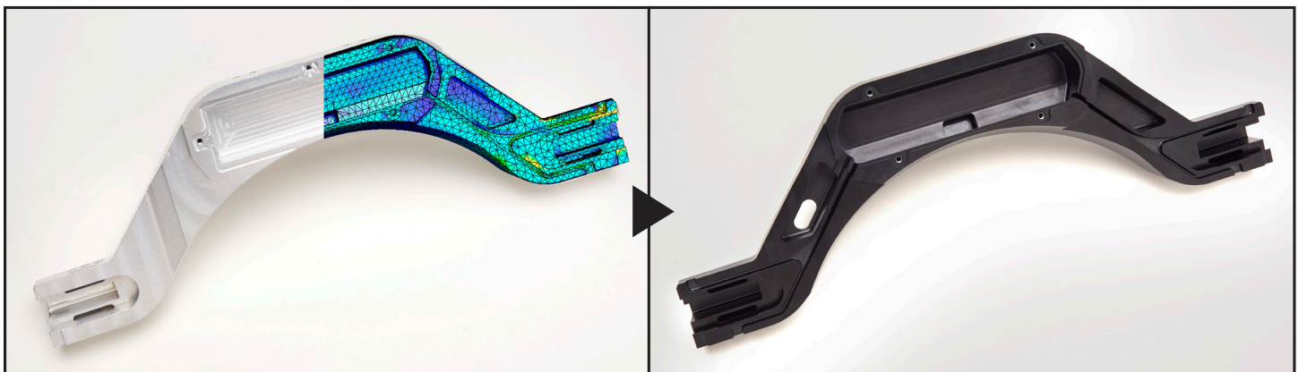
Aluminum bracket with half FEA analysis (left) and KyronMAX final molded part (right). The FEA analysis is used to translate a metal part into a lightweight plastic molded part, while matching or exceeding the strength and stiffness of the original metal part.
