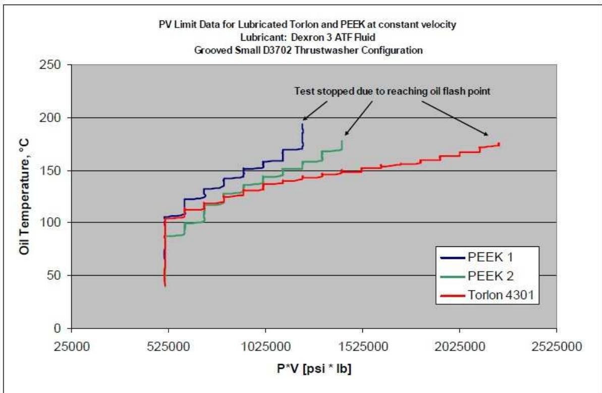
Photo caption 8: PV Limit Data for Lubricated Torlon and PEEK at constant velocity
